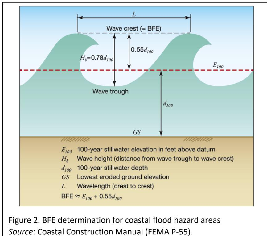
Figure 2. BFE determination for coastal flood hazard areas
