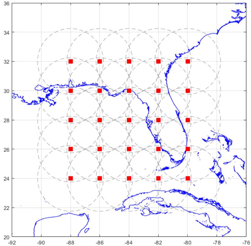
**Figure 2-2. Locations of simulation circle centers showing extent of 250 km sample circles near Florida.**
