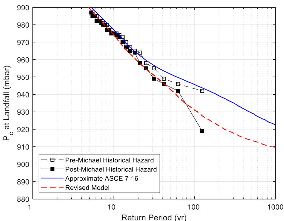
**Figure 2-1. Hurricane hazard curves (as defined by central pressure at landfall) in the Florida Panhandle region. The historical hazard before (open black squares) and after (filled black squares) Hurricane Michael and the modeled hazard before (solid blue line) and after (dashed red line) mode updates were performed are shown for comparison.**
